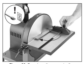
Figure 26. Squaring miter gauge to disc.
